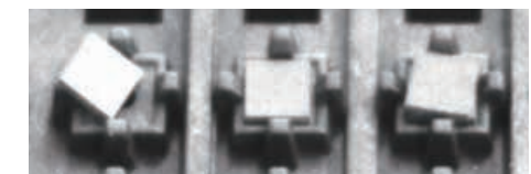
▲ Chip lead bent ▲ PCB assembly inspection
